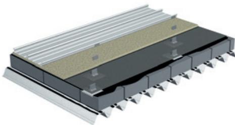
The FOAMGLAS® slabs are bonded to different substructures using either a cold-bonding agent or hot bitumen. In order to attach the compound clips, the galvanized steel claw plates are inserted under heat in a fixed installation plan taking into account the respective roof geometry. The compound clips are installed on the claw plates using the recommended fastening elements.
