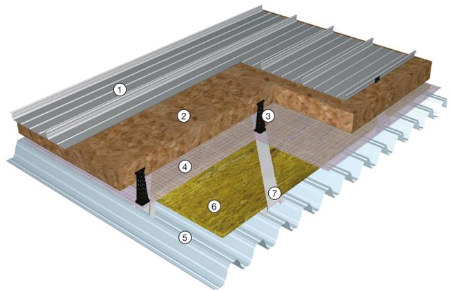
**Kalzip standing seam on Kalzip structural decking with top hat sub purlins**
