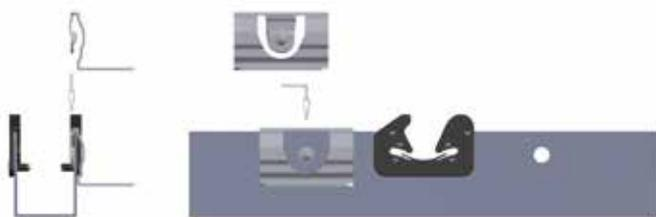
Number and arrangement for the fastening of lesene: approx. 1.5 units/m (arranged offset)
