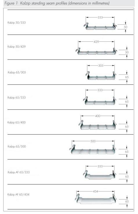
1.3 Profiles are manufactured from aluminium alloys in various finishes to BS EN 485-1 : 2008 and BS EN 1396 : 2007:
